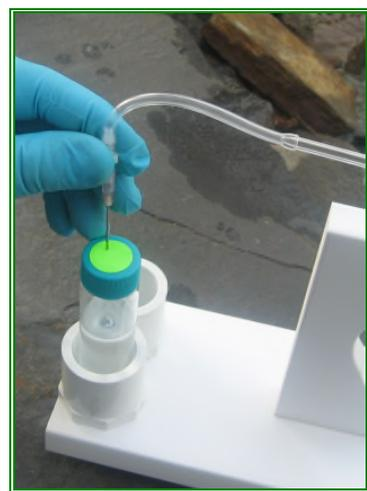
5. Connect a new extraction needle assembly to the colorimetric tube by sliding the open end of the vinyl tubing over the broken end of the colorimetric tube. This step must be completed before inserting the needle into the VOA (Prior to step 6).
