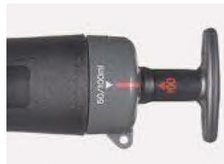
13. If no color-change reaction is visible or if the color reading is less than 1.5, rotate the pump handle ½ turn and pull the handle out to lock in the 100ml position.
