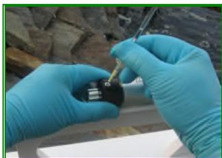
3. Break both ends of the colorimetric tube using the tip breaker on the piston pump.
