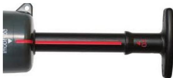
14. Continue the 100ml purge until the flow cycle is complete. Note: Flow is complete when the end-of-flow indicator (located on the back of the pump handle) returns to its full brightness.
