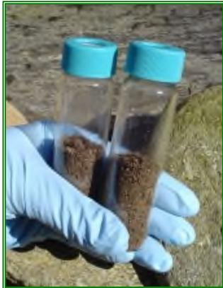
**IMPORTANT NOTE:** The VOA vials containing the solid sample media and “clean” water must contain an air-filled headspace to accommodate purging. The caps must be tightened sufficiently to prevent loss of CVOHs during the time between sample collection and analysis (which includes the heating process) and to prevent air leakage during the purging process.
